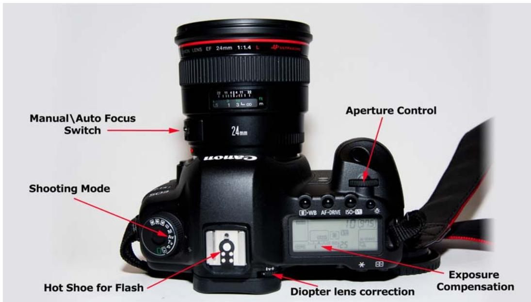
**3. Exposure meter** - most new cameras have several types of metering systems - they all measure light reaching your digital sensor. The choices include: 1) multisegment also called Matrix, evaluative, or honeycomb 2) Center weighted and 3) spot meter. Spot metering is used in difficult lighting or backlit situations and requires the most skill to use properly. I recommend you set your camera to use Matrix metering most of the time (i.e. 99% of the time).
